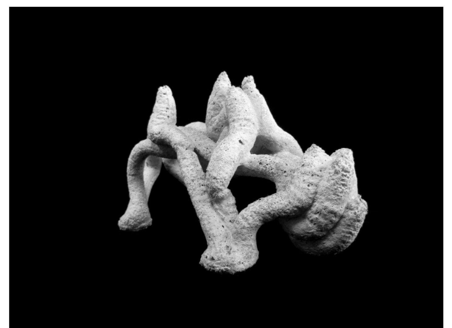
Internal skeleton by I3DCP (cast in lime suspension), block 2
