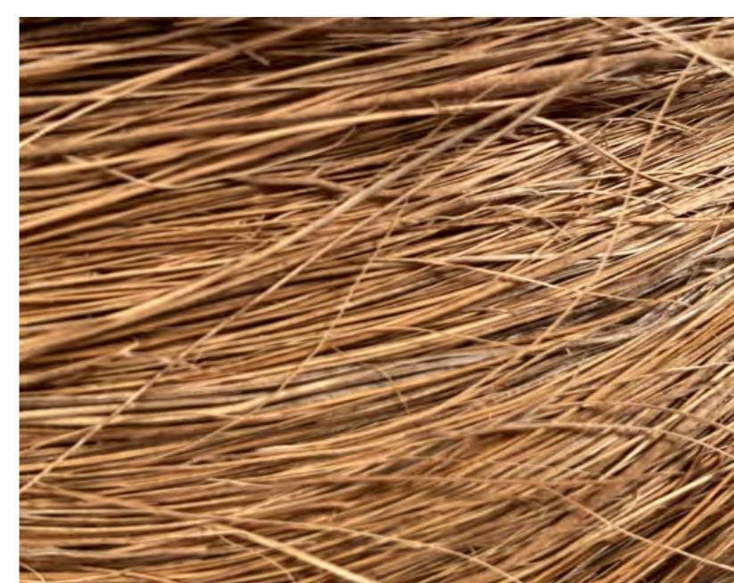
Coir fibre (diameter 0.1-0.5 mm)
