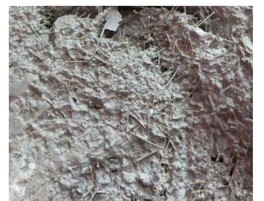
Coir fibre in "muscle" of insulation block)
