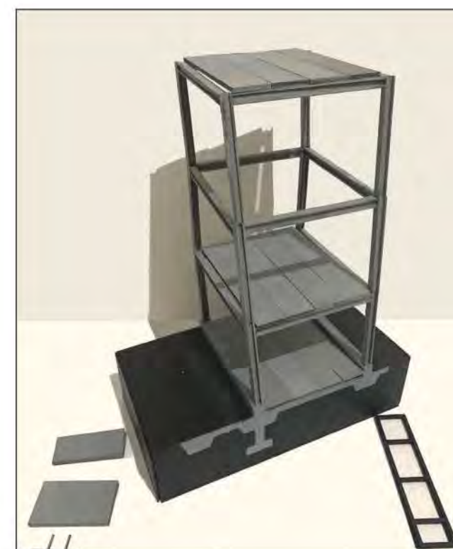
1:20 Fragment - Connection between existing Concrete Column and Salvaged Timber
