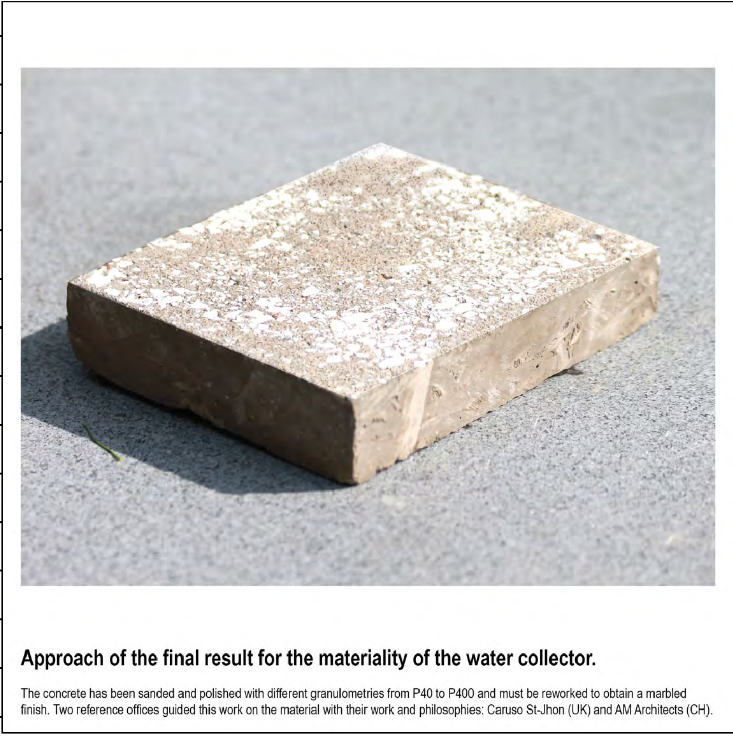
Device detail. A research into constructive detail and the materiality contributes to this phenomenology . The concrete of the collection tray is made of crushed marble (collected in situ); a dry assembly of the grating and a minimum anchoring of the structure in the collection tray; a staircase whose stone steps are inserted on a concrete block made of crushed bricks.
