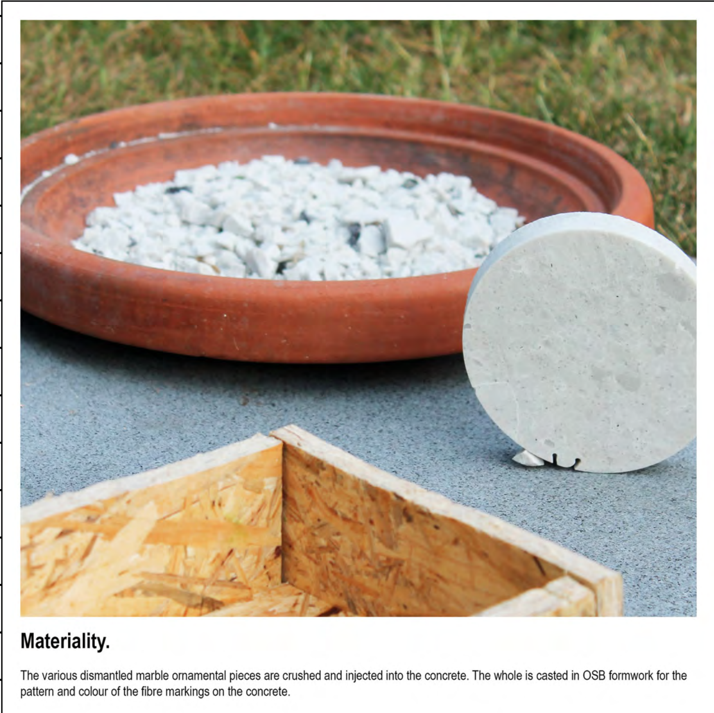
Regenerating cultural identity through materials (cross-section). The water collection tank is a phenomenological device reflecting the immaterial and singular memory of the place by means of a waterproof concrete incorporating fragments of marble decorations . The whole is visible through the wooden grating and is related to the codified constructional techniques, the old oven and the landscape/collective space .
