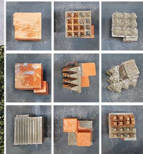
Making: Test Pour with different surface qualities like: sponge, egg crate, corrugated plastic and woodfibre boxes.
