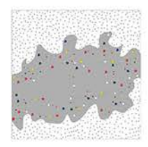
04. Remove timber formwork when plaster layers have set. Begin to remove soil layers. Then proceed to chisel and brush the remaining soil, using knitting needles, a brush & a screwdriver.
