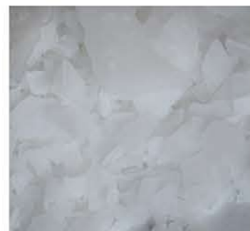
Magnesiumchloride flakes (MgCl2) are dissolved in water before mixing with CCM to create MOC.
