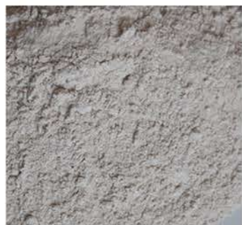
Caustic calcined Magnesiumoxide (CCM) burnt at 800°C suits best for MOC usage because of its high reactivity.
