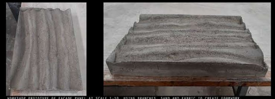
WORKSHOP PROTOTYPE OF FACADE PANEL AT SCALE 1:10, USING BRANCHES, SAND AND FABRIC TO CREATE FORMWORK.
