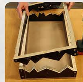
PICTURE 8 - Lower and top part of mould fit perfectly
