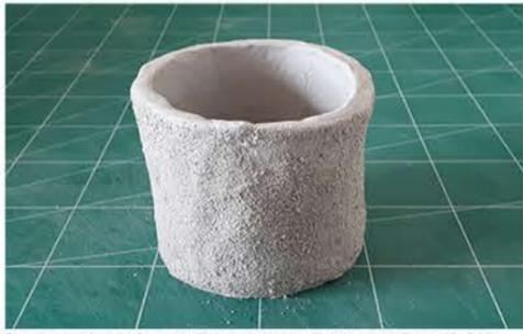
Recast concrete pot using reconstituted aggregate with layer of granite sand to finish.
