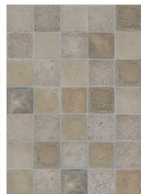
Recycled cast concrete cladding for Sarsfield House, variety of colour and texture shown.
