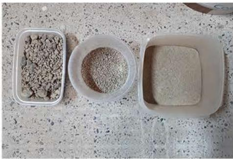
Granite aggregate concrete, crushed and returned to its constituent aggregates.
