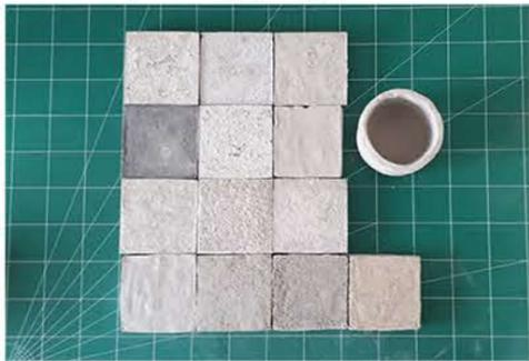
Recast concrete using reconstituted aggregate, Small gaps for mortar between.
