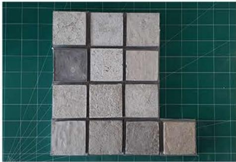
Recast concrete using reconstituted aggregate, large gaps for mortar between.
