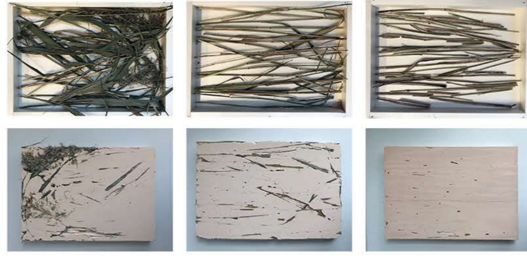
MATERIAL EXPERIMENTS WITH DIFFERENT PATTERNS OF REED WITHIN PINK PIGMENTED CONCRETE
