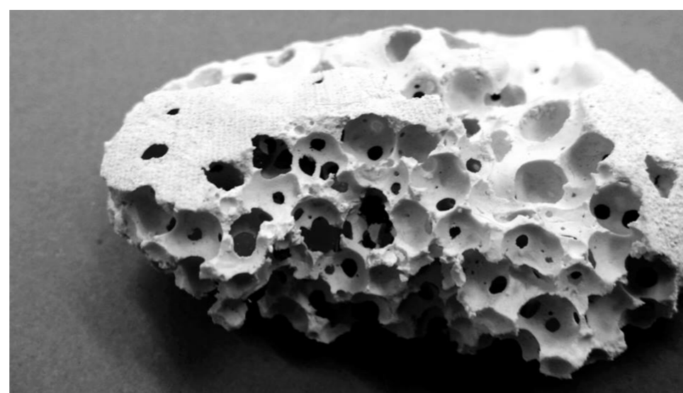
small scale material investigations with concrete using water beads to form voids
