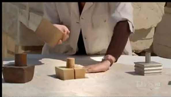
Parthenon wooden drums connectors (left) and replaced titanium connector (right), Athens, Greece
