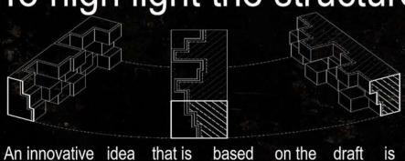
An innovative idea that is based on the draft is a three-dimensional printable formwork panel. The surface of the panel can be optionally and highly complex offset with pigments. During the formwork process, it creates complex structures and at the same time a long-lasting economic and highly differentiable pigmentation of concrete surface.
