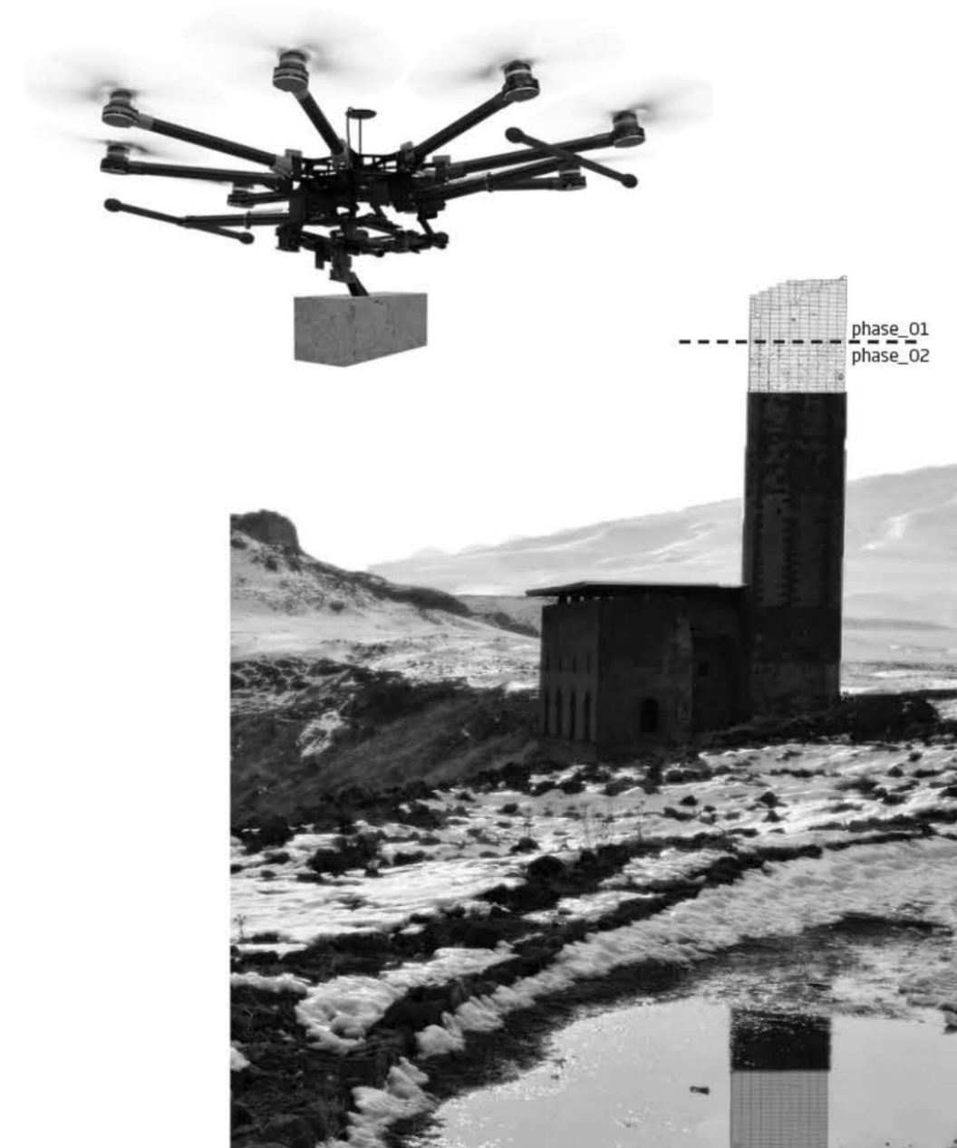
scen(e)ario_03 : con/drone system could be used in restoration of old structures. Most of drones could carry the prefabricated concrete bricks, and some drones could connect them or hold the formwork. In time, new parts will become green, and differentiate from old structure. Understanding the new installed parts is one of the principles of a good restoration.
