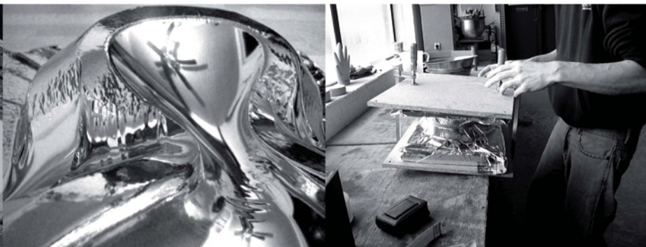
4. vacuum-formed package | to avoid vacuum between concrete and formwork | for clean finishing without special treatment |
