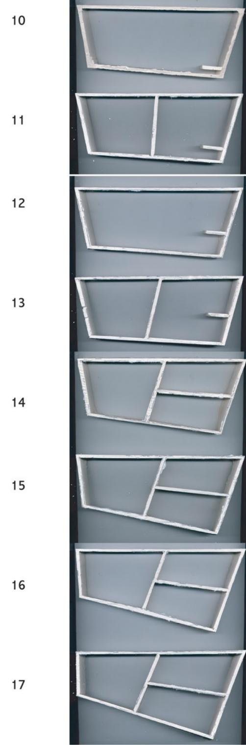
The images illustrate the seventeen sections used to create the form of the visitor centre. Subtle changing and morphing of the section create complex interesting internal spaces and volumes. Once the sections have been assembled and post-tensions they form an efficient beam capable of spanning the ravine where the project is sited.
