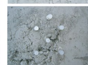
DEVELOPMENT OF GLASS-FILAMENT+ ACRYLIC WALL - ESTABLISHING THE NEED FOR SUPER PLASTICISERS, TO FLOW AROUND THE RODS
