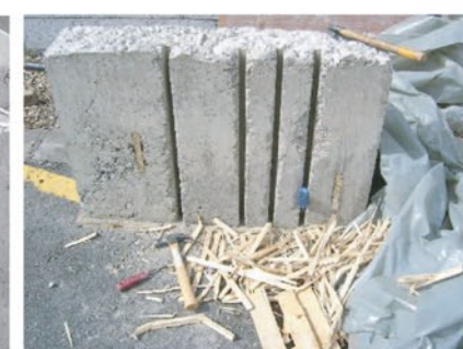
SOUND POCKET DEVELOPMENT - WHERE SOUND FLOWS THROUGH PUNCTURED + PERFORATED WALL STRUCTURE
