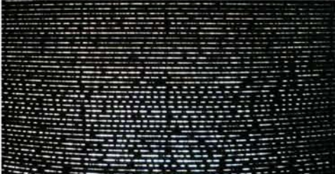
Work-up of optical-fiber-concrete
