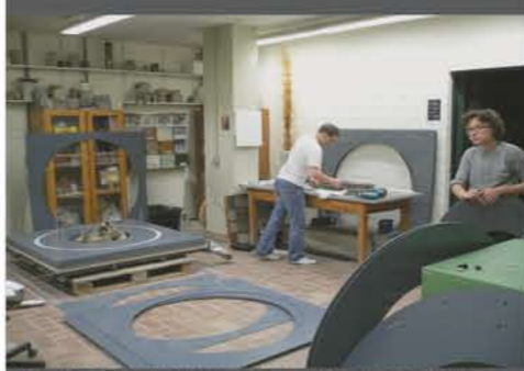
Work-up of the form-work with inserted optical-fiber-textile in all layers
