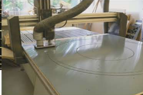
Production in form-work (CNC-milling machine)
