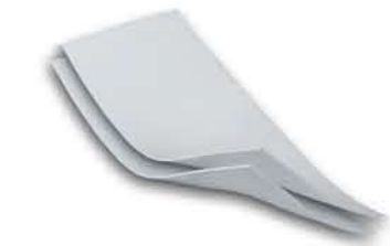
Thermoplastic polyethylene (PE) panels can be deformed at temperatures starting from 110°C and easily welded together.
