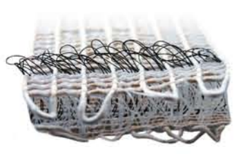
3-dimensional meshworks serve as reinforcement. Glass fibers in the top and bottom chord take over the tensile loads. Thermoplastic fibers separate the two glass fiber layers from each other. Monofilaments keep the meshwork in place.
