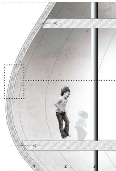
1 Thermoshape sandwich element filled with concrete (thermoplastic layer removed) and connected with the frame construction with façade anchors 2 shiny concrete surface 3 frame construction
