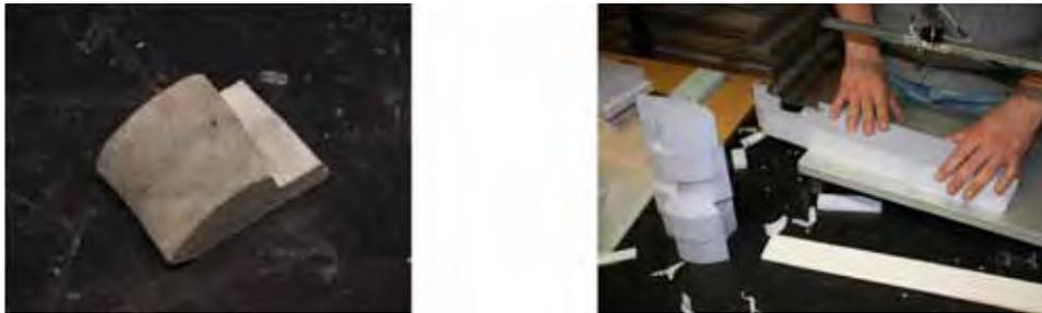
We have made extensive studies into the ratio of concrete mixes to create a formula that can float as well as ability to retain the texture of its fabric formwork. The potential of this floating infrastructure to produce energy is opportunistic and is making use of existing technologies being developed on the west coast of Ireland.
