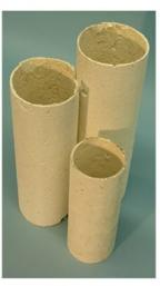
We decided to add a water based compound admixture to the cement to allow us to make the material less dense, thinner and less brittle. Our first thought was to use gelatine as an admixture as it also reacts with water allowing it to set. Our investigations lead us to look at applications where gelatine is used.
