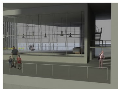
Another wall in the middle (1), who is connected with the other wall in the middle (2) and the horizontal plates (3). This creates an extension of the wall, but one level higher. The passage (4) under it is hung up to this vertical plate(1) an generates an open space (5) without columns on the level below.
