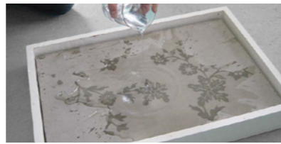
Figure 1: Smart concrete; the concrete unveils figures as soon as it comes into contact with moisture (source: http://traces.co.kr/tc/236 )
