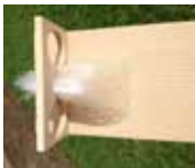
/ The formwork process. 12 mm MDF with 1,5 mm drilled holes for the fibers. Top lid with pouring holes and holder for the fibers.
