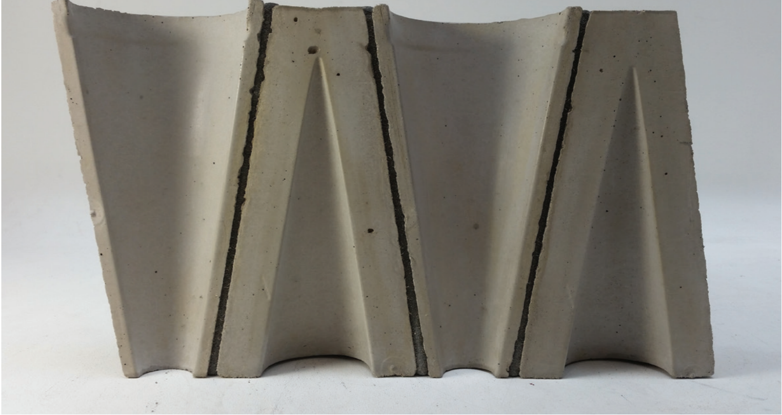
8. The Sand is brushed out and leaves recessed seams. The sand leaves a texture to the seams in contrast to the smooth concrete Cones.
