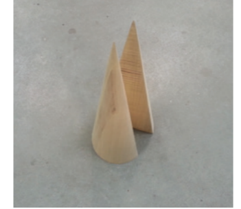
1. Wooden Cone, made on a bench lathe.
