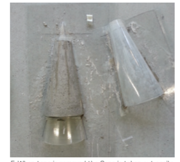
5. When tape is removed the Cone is taken out easily due to the applied wax.
