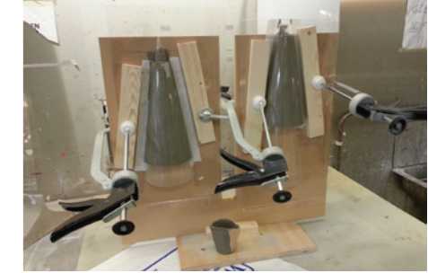
4. Molds Filled with fiber reinforced concrete.
